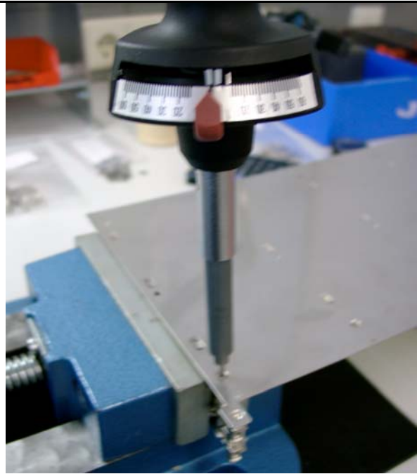
Photo 2= Trial with die-cast strut part no.: 60849-022. Measurement performed with STAHLWILLE torque tester.
