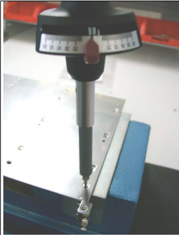
Photo 3= Trial with die-cast strut part no.: 60849-023. Measurement performed with STAHLWILLE torque tester.
